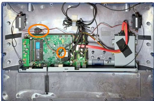
Photo: Position of the button cell battery and the connector on the mainboard with the computer housing open.
