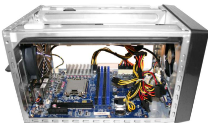
Photo without chassis cover, drive rack and heat-pipe cooling
