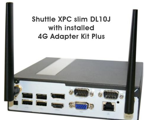
4G Antennas with Cables
