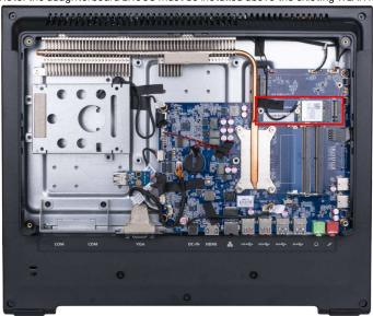
**2.** Install the daughterboard (LN008) into the M.2 slot and secure with the screw.
