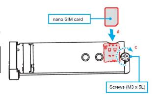
**4.** Please install an 5G (or 4G) module in the relevant slot on the daughterboard (LN008), then tighten the screw with bolt firmly. As shown, connect the four antenna cables to the 5G module (two antenna cable to the 4G module).
