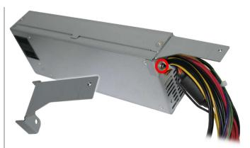
Push the cables of the power supply through the internal housing opening as shown in the picture.
