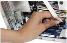
8 Make sure that the marked lead of the ribbon cable and the marking on the mainboard are on the same side.
