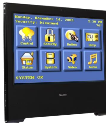
Control Surveillance, Home Automation, Control device
