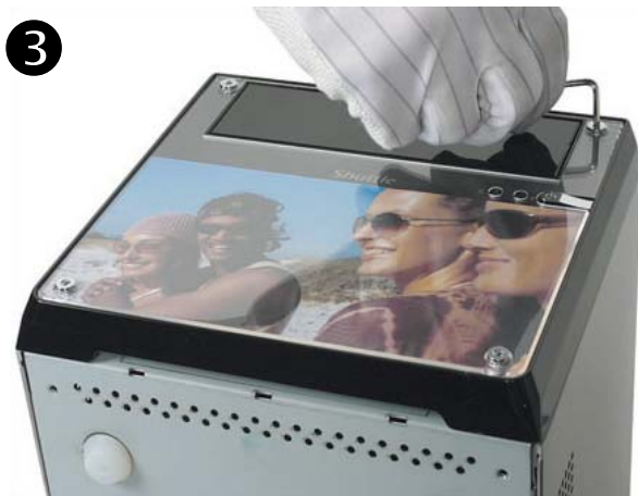
3 Align and correspond the transparent glass and new image to screw holes on the front of the machine. Carefully screw back the four screws.
