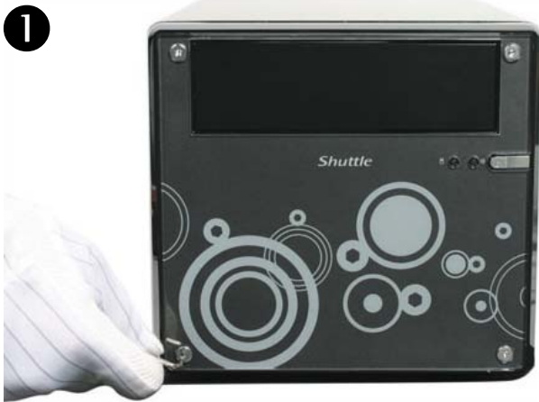
1 Unfasten the front panel by removing the four screws. Remove both the transparent glass and the image.
