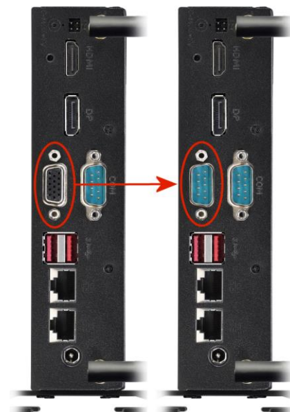
Shuttle XPC slim DS10U before and after the installation of one PCP11 adapter
