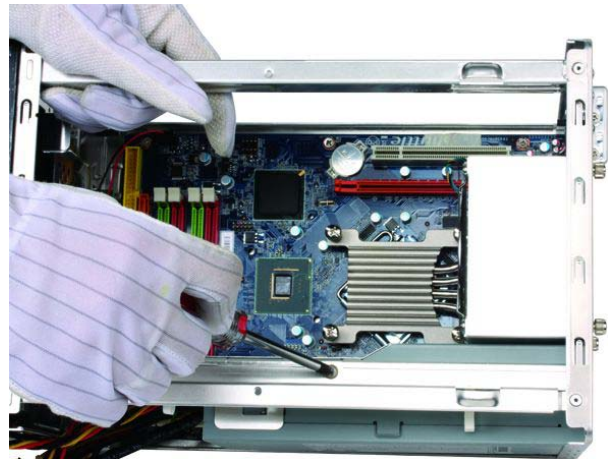
④ Finally, secure again from top with Phillips head screw.
