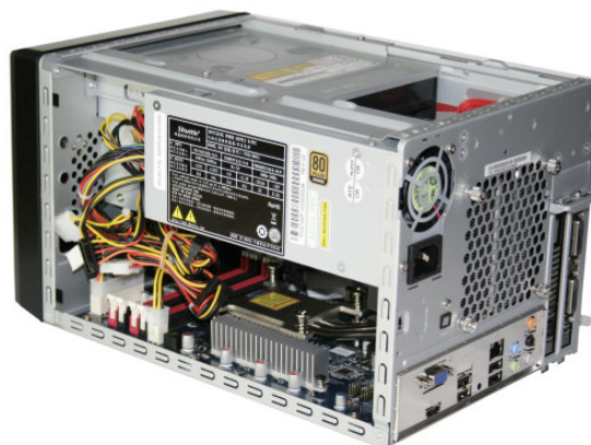
③ Attach the 20-pin ATX and 2x2-pin (or 1x4-pin) power supply plugs to the mainboard.
