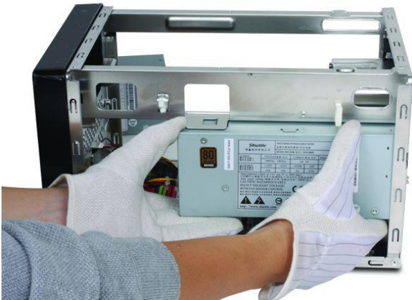
① Place the power supply in position. Secure from the back with three Phillips head screws.
