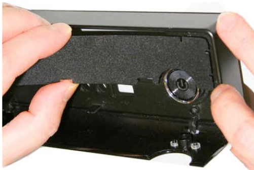
Installation of the self-adhesive mylar
