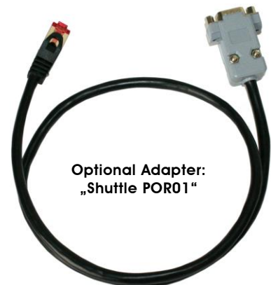
Shuttle Accessory POR01 Matching COM port adapter converts RJ45 to D-Sub ports (optional, not included in delivery)
