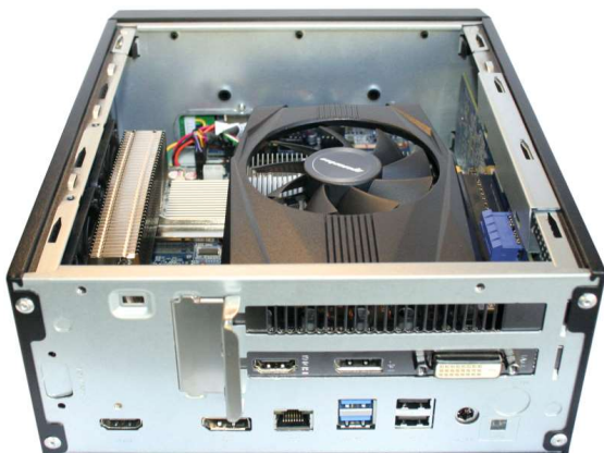
Shuttle XPC slim Barebone XH510G2 with powerful graphics card installed
